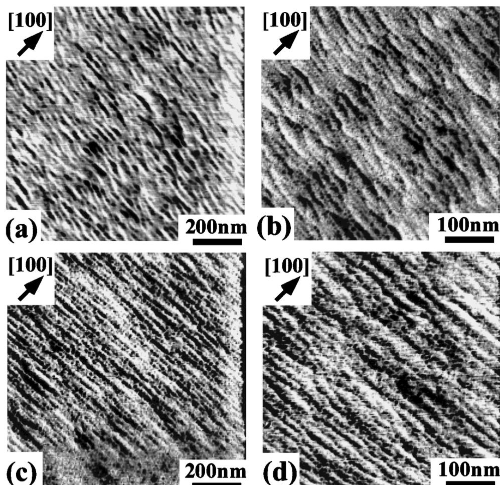
Fig. 1. STM images of the surface of vicinal GaAs(001)-[100]2° annealed in H<sub>2</sub> ambient for 550°C for 20 min, (a) and (b), and 650°C for 10 min, (c) and (d). The scale is 1000 × 1000 nm for (a) and (c), 500 × 500 nm for (b) and (d).
