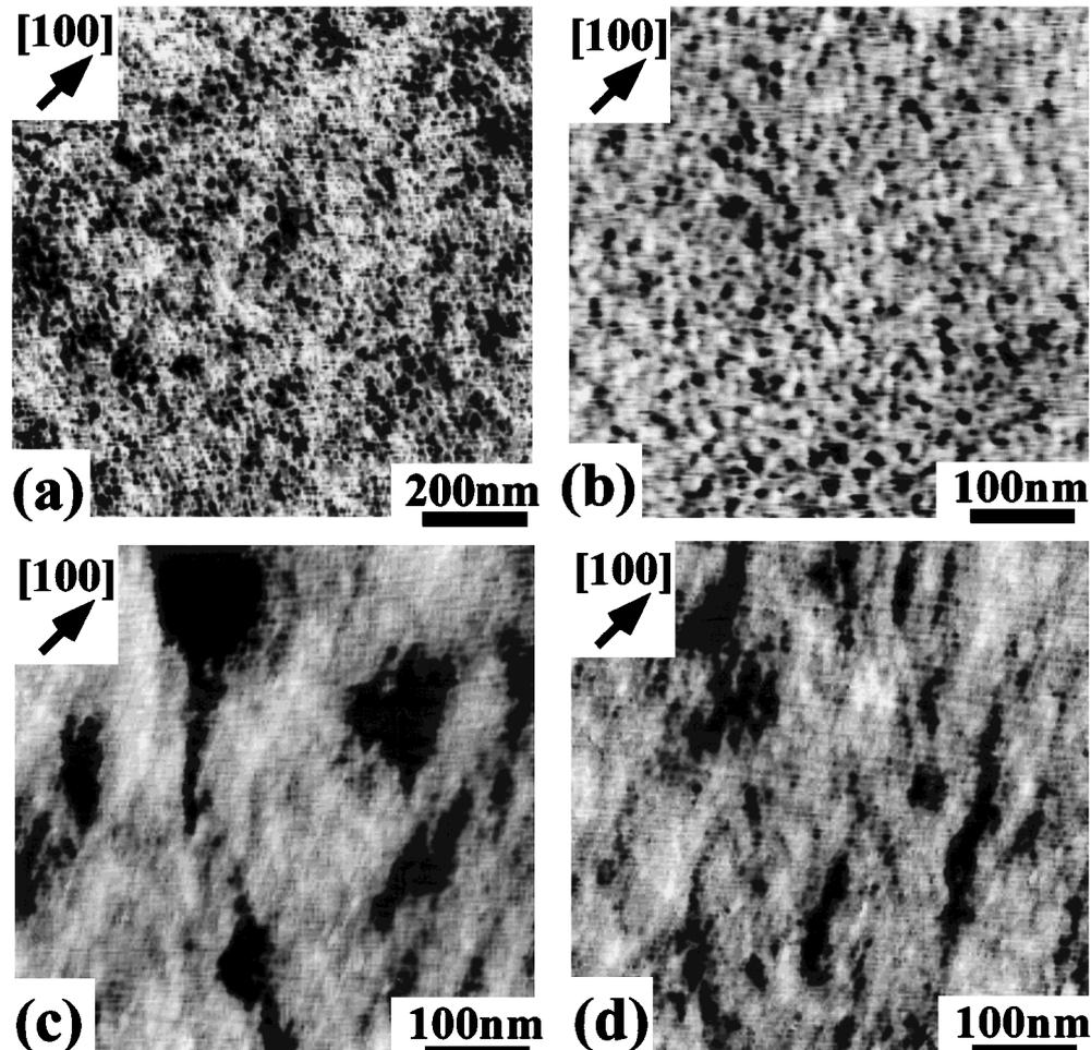
Fig. 2. STM images of the surface of vicinal GaAs(001)-[100]<sup>2°</sup> annealed in N<sub>2</sub> ambient for 550°C for 10 min, (a) and (b), and 550°C for 20 min, (c) and (d). The scale is 1000 × 1000 nm for (a) and (c), 500 × 500 nm for (b) and (d).
