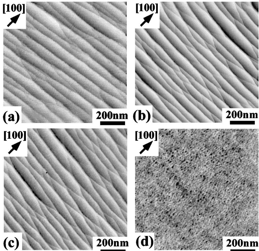
Fig. 3. STM images of the surface of vicinal GaAs(001)-[100] $2^\circ$  annealed in AsH<sub>3</sub> and N<sub>2</sub> ambient for 650°C (a) and 700°C (b) for 10 min and surface annealed in AsH<sub>3</sub> and H<sub>2</sub> at 700°C for 10 min (c) and just after chemical etching (no annealing) (d). Scale of all images is 1000 × 1000 nm.
